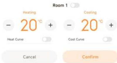
Room temperature control (Heating/Cooling Target room temperature in Zone 1)
