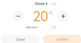
Circuit water temperature control (Target water temperature in Zone 2)
