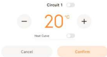
Circuit water temperature control (Target water temperature in Zone 1)
